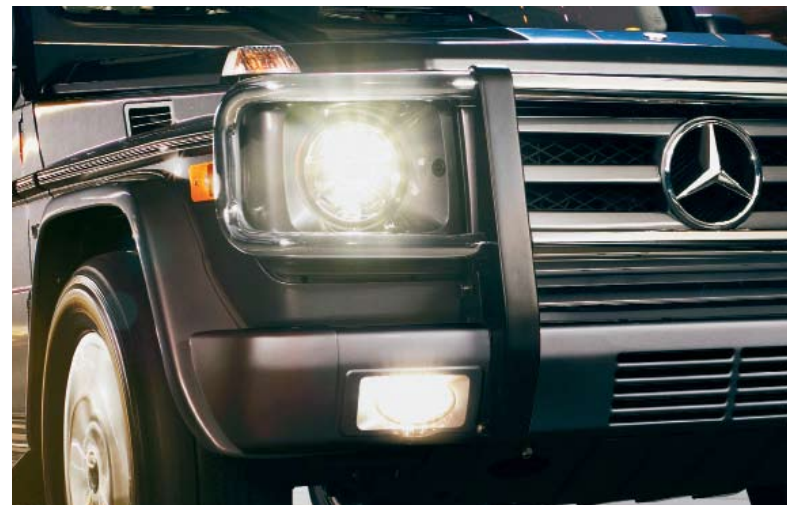
Bi-Xenon headlamps with corner-illuminating front fog lamps
