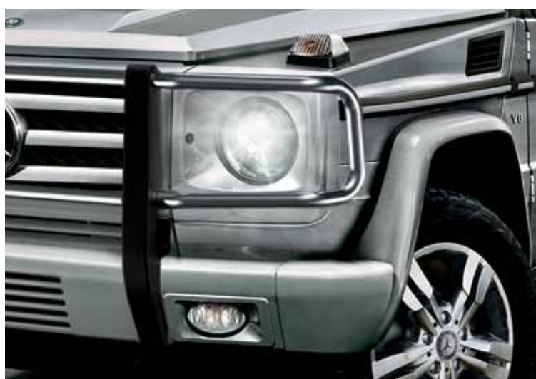
Bi-Xenon headlamps with corner-illuminating fog lamps
