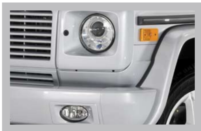
Bi-Xenon headlamps and corner illuminating fog lamps
