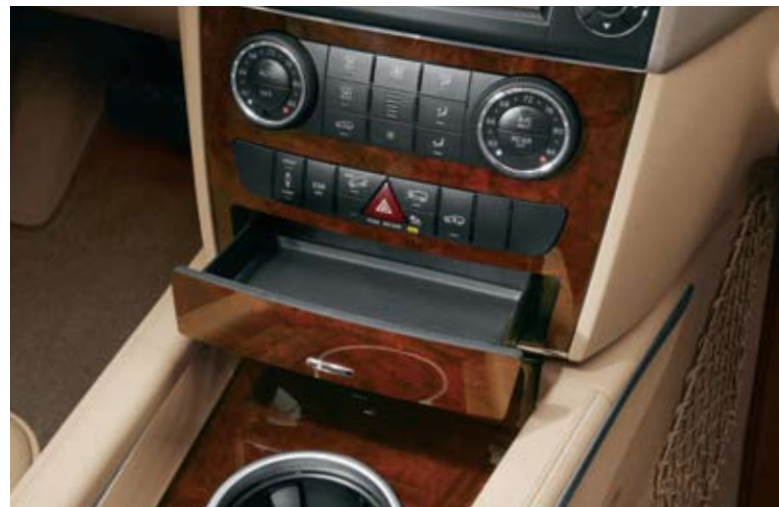
Wood storage tray located below climate control
