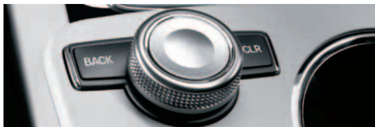
Central controller with 5-inch display
